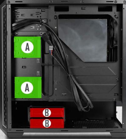
Flexible hard drive mounting system boasts enough mounting brackets for up to four 2.5" SSD
